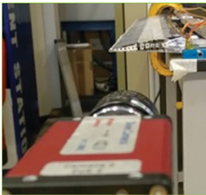
Fig. 6: Imetrum camera tracking chordwise points
