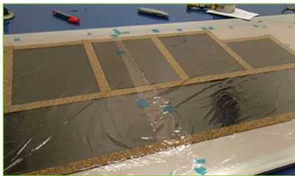
Fig. 2: Manufacturing the carbon fibre spine using a standard vacuum bag and autoclave curing process
