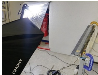
Fig. 4: FishBAC wing during the static structure test. Extra light sources are added to increase the visibility of target points
